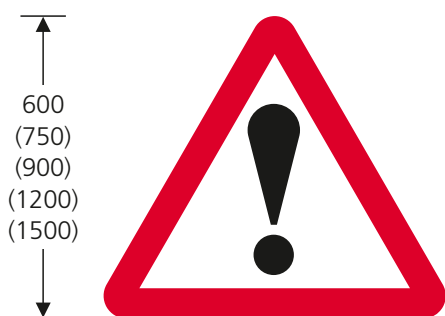
562 Other danger ahead
