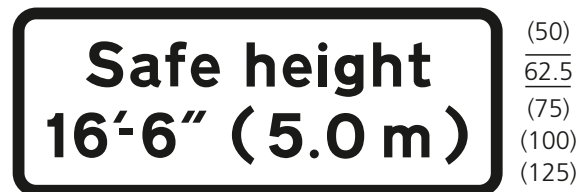
780A Safe height beneath cable
