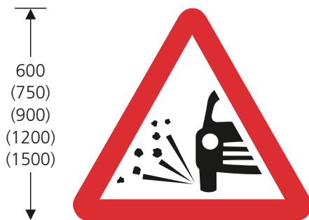
7009 Loose chippings on road ahead
