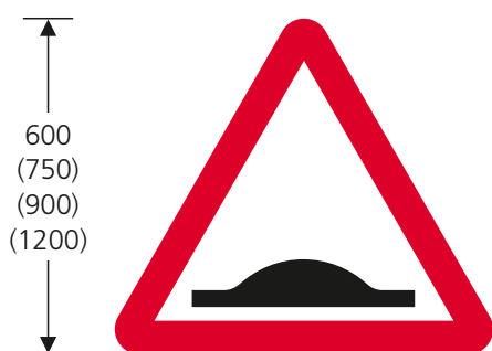
557.1 Road hump or series of road humps
