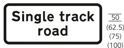
519 Road wide enough for one line of vehicles only
