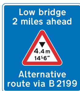
Figure 7-3 Signs on approach to an arch bridge with a diversionary route
