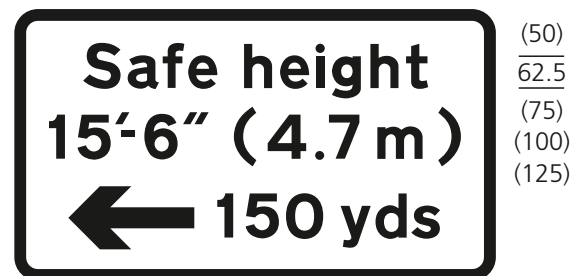
780.1A Safe height beneath cable in direction and at distance indicated
