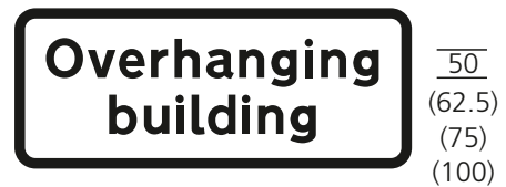
530.1 Building overhanging part of carriageway
