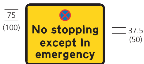
642.3 No stopping in lay-by except in emergency
