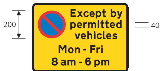
640.4 Waiting prohibited in a designated off-highway loading area except by permitted vehicles
