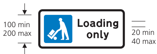
660.4 Part of the carriageway reserved for loading and unloading
