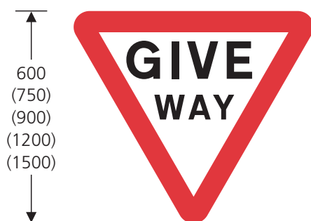
602 Junction controlled by a GIVE WAY sign
