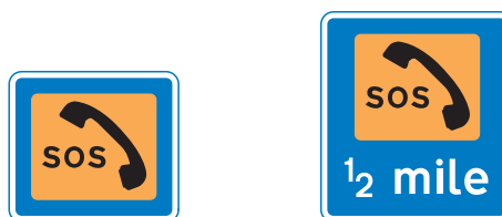
Location of emergency lay-by with telephone
